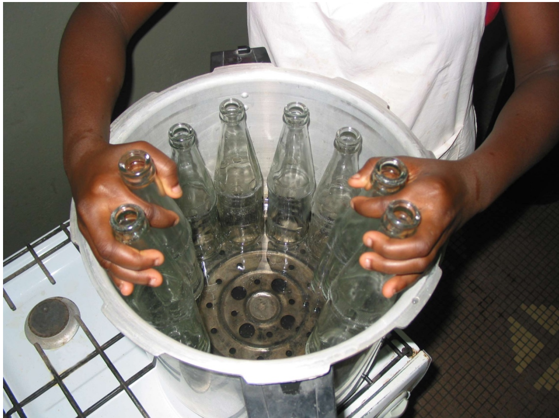
Source: Université d'Abomey-Calavi (2015) – Sterilizing glass bottles in boiling water before bottling
