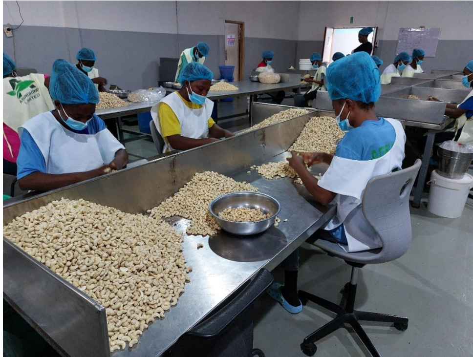
Fig. 18: Manual final inspection of the cashew nuts by female workers.
