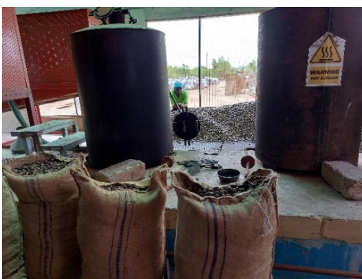
Fig. 16 (right): In the first step the cashew nuts, still in their shells, are heated at the factory to make the shells easier to remove.
