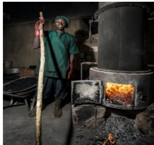
Use of cashew shell for power generation in the steaming process. Source: ComCashew
