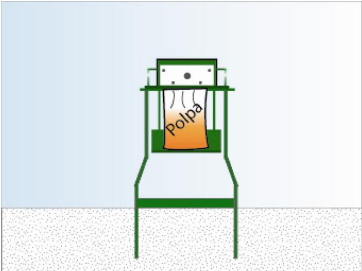
Figure 8 – Hand-operated sealer for cashew pulp
